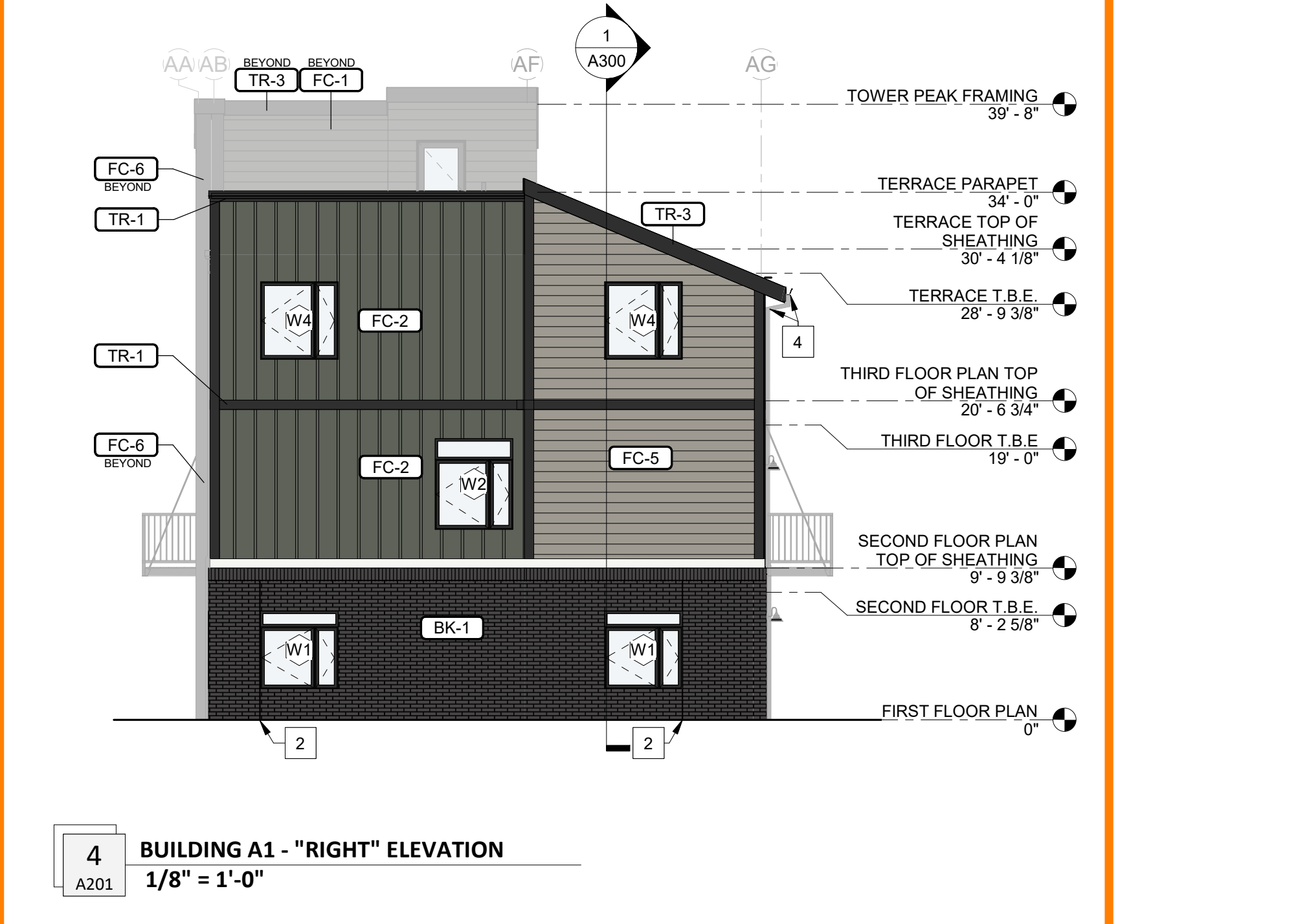
4 BUILDING A1 - "RIGHT" ELEVATION 1/8" = 1'-0"
