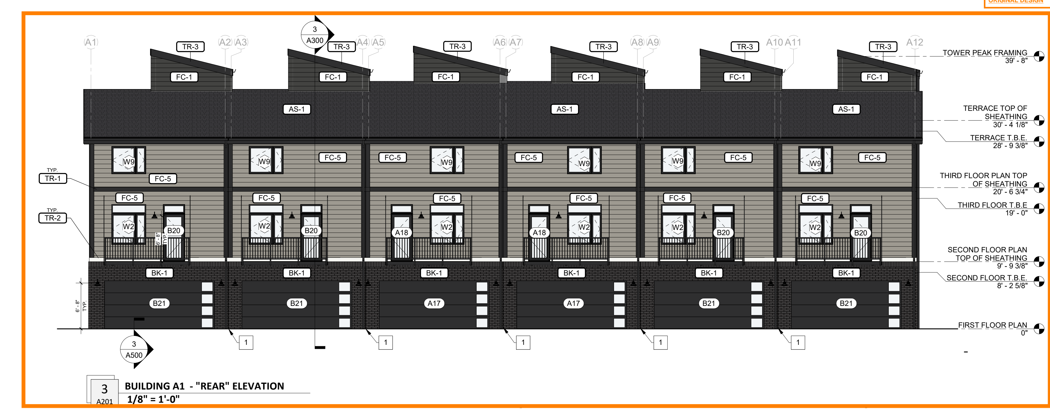
3 BUILDING A1 - "REAR" ELEVATION 1/8" = 1'-0"
