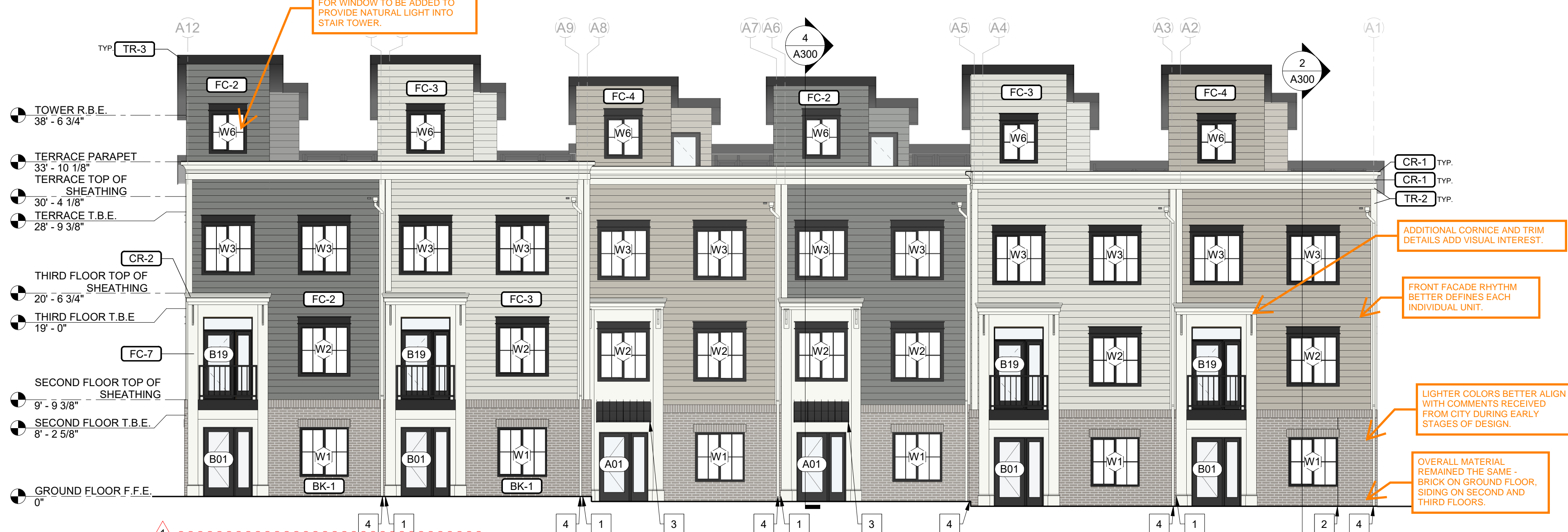
1 A201 BUILDING A1 - "FRONT" ELEVATION 1/8" = 1'-0"
