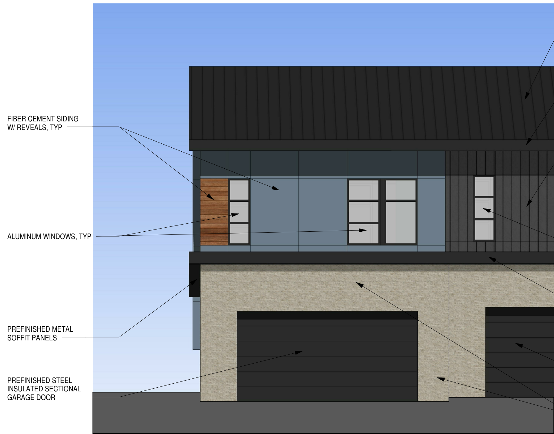
TYPICAL REAR AND GARAGE ENTRANCE ELEVATION
