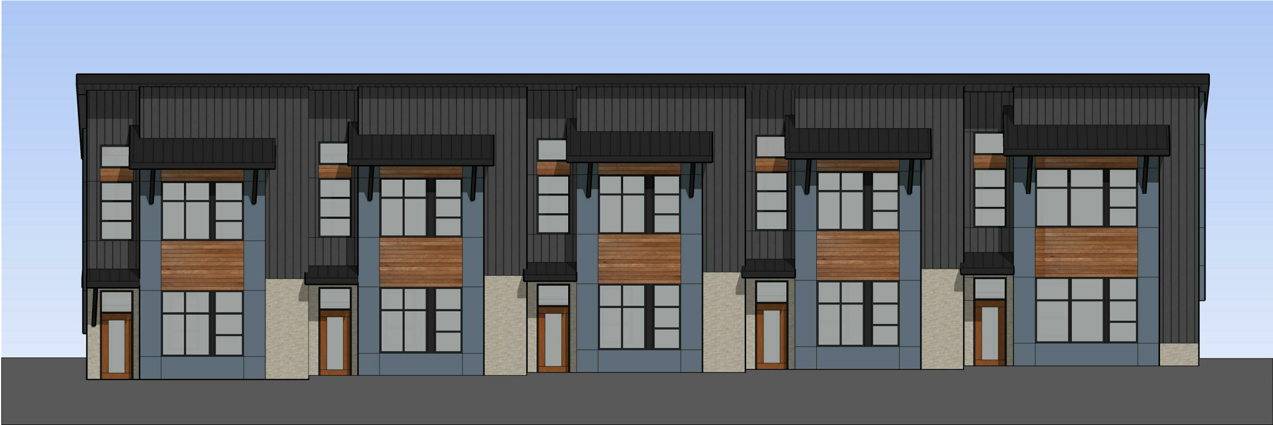
SOUTH OVERALL AND TYPICAL 5-TENANT FRONT ELEVATION
