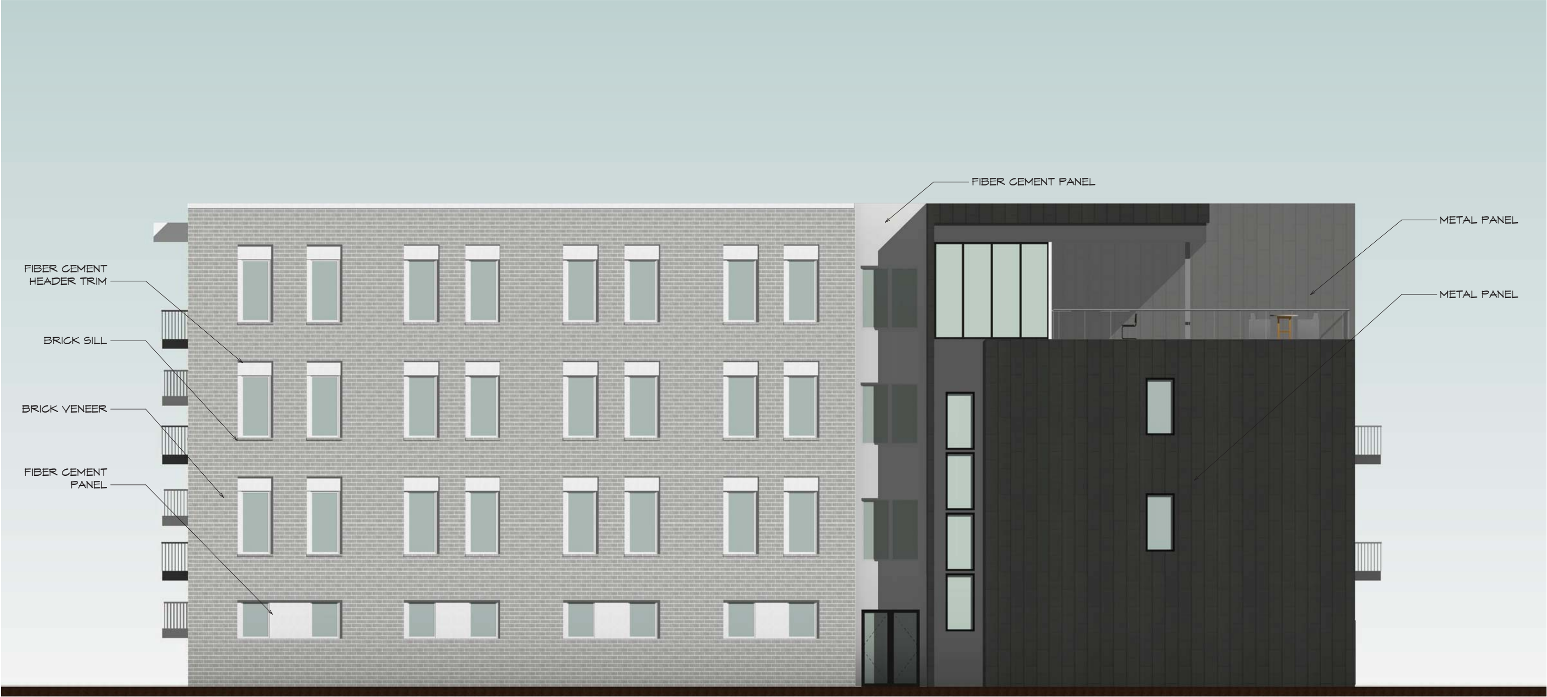
MIXED - USE BUILDING : SOUTH ELEVATION
