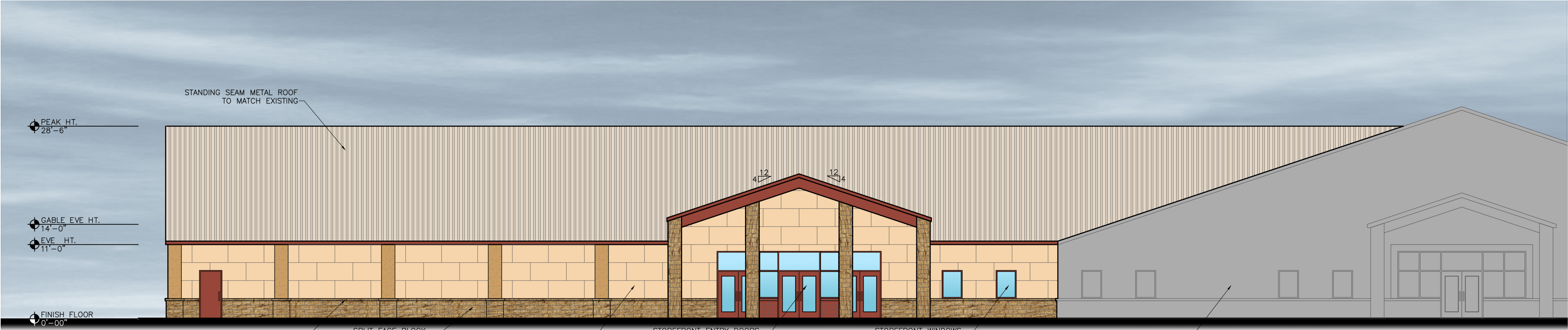
1 FRONT ELEVATION SCALE: 1/8" = 1'-0" SPLIT FACE - 26% HARDIE PANEL - 58% STOREFRONT - 11% EFIS - 5%
