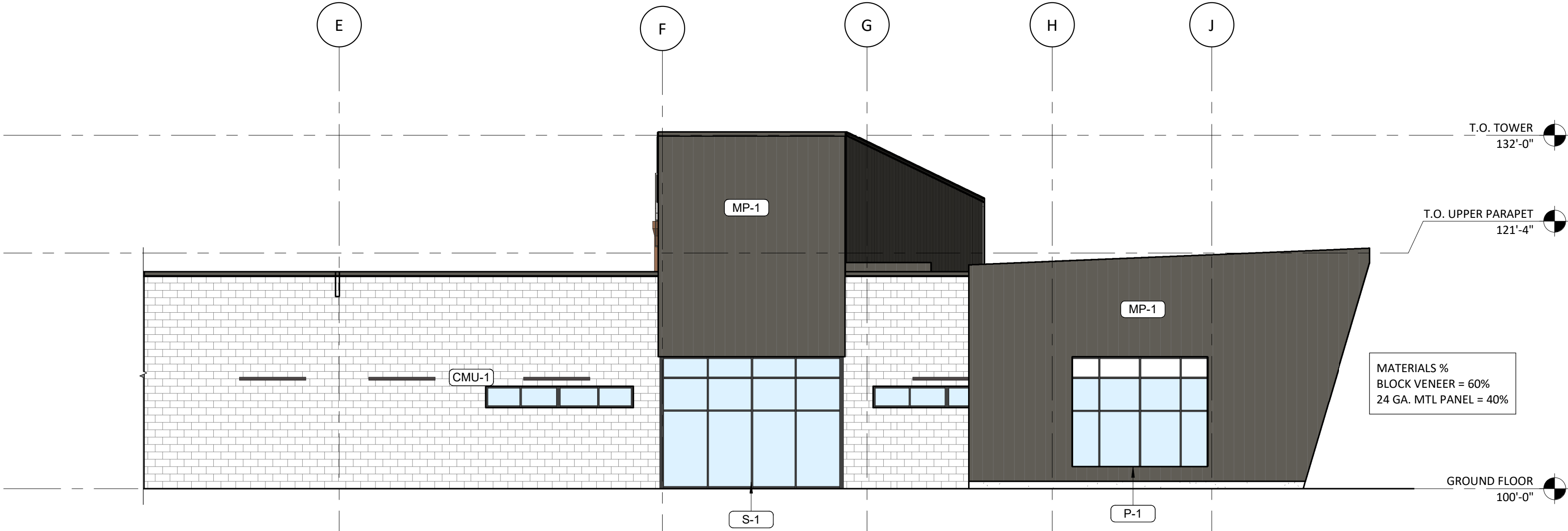
1 BANK ELEVATION - SOUTH 1/8" = 1'-0"
