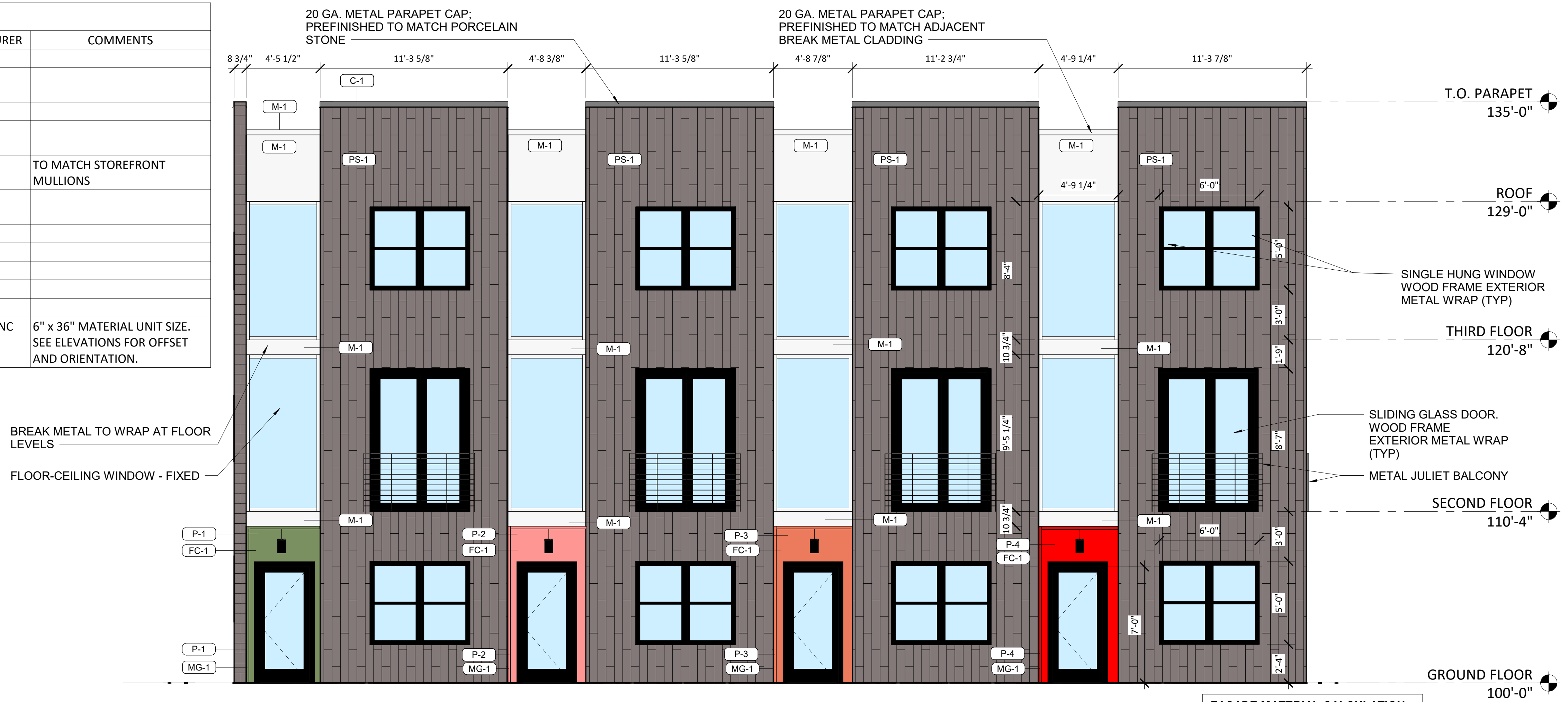
2 FRONT ELEVATION (STREET FACING) 1/4" = 1'-0"
