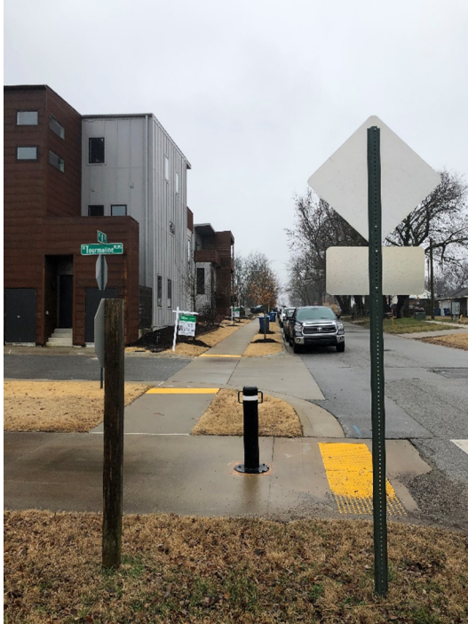
No Stop Control on SE D St. Parallel parked cars are within sight triangle.
