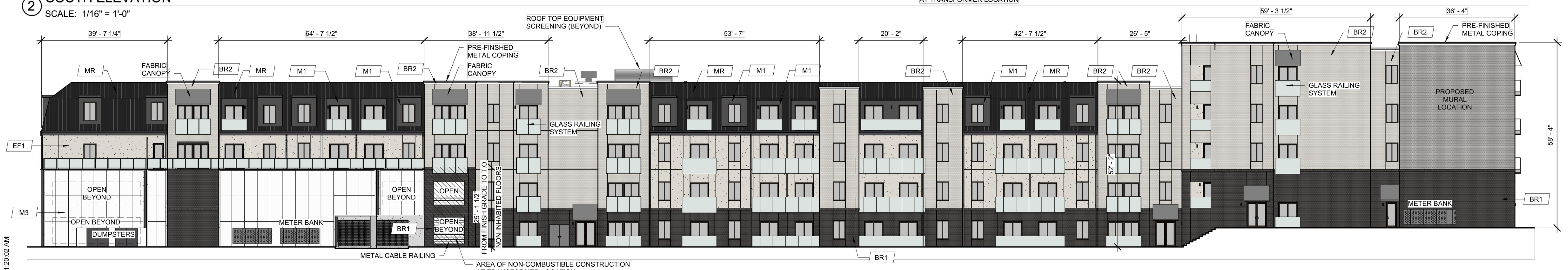
1 NORTH ELEVATION SCALE: 1/16" = 1'-0"
