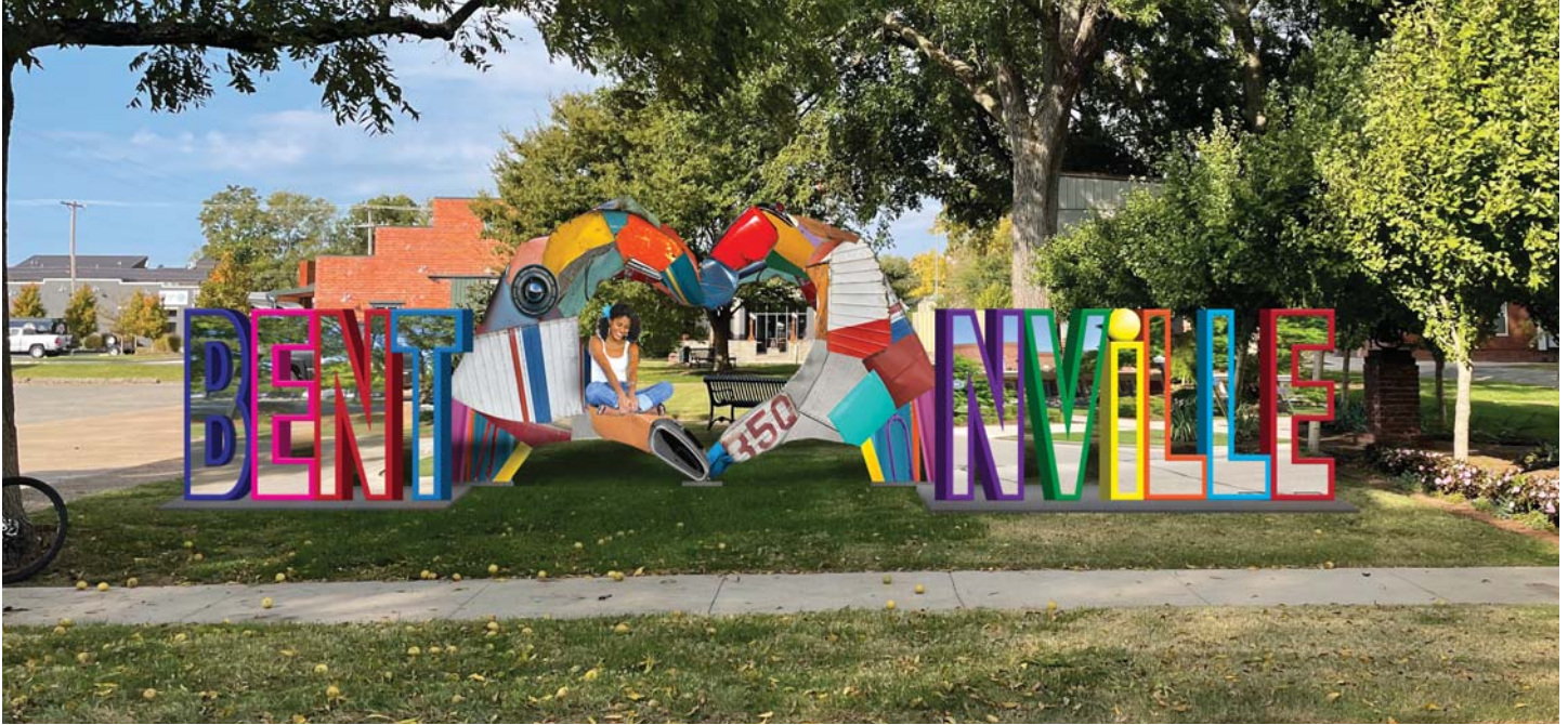
BENT♥NVILLE Option #3 featuring acrylic mirror clad 1/8" steel filling the letters.
