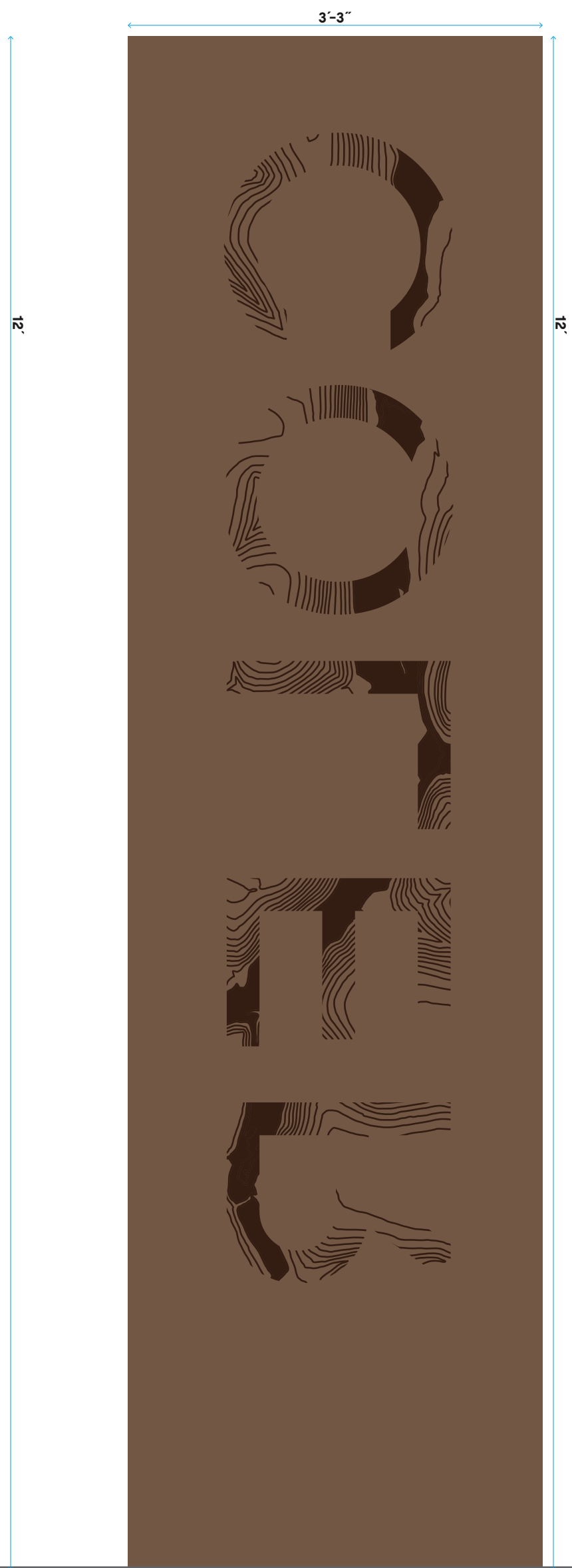
3'-3" x 12' 18" subsurface north gateway and south gateway / 3rd street metal slab with cut through typography back
