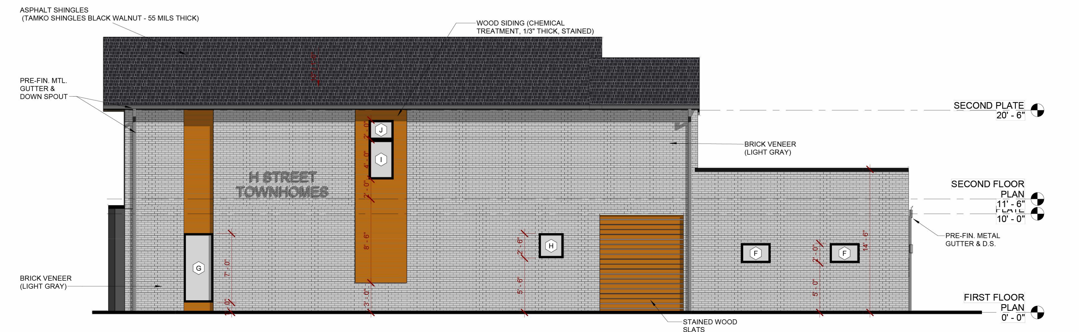
3 SIDE ELEVATION - NORTH 3/16" = 1'-0"
