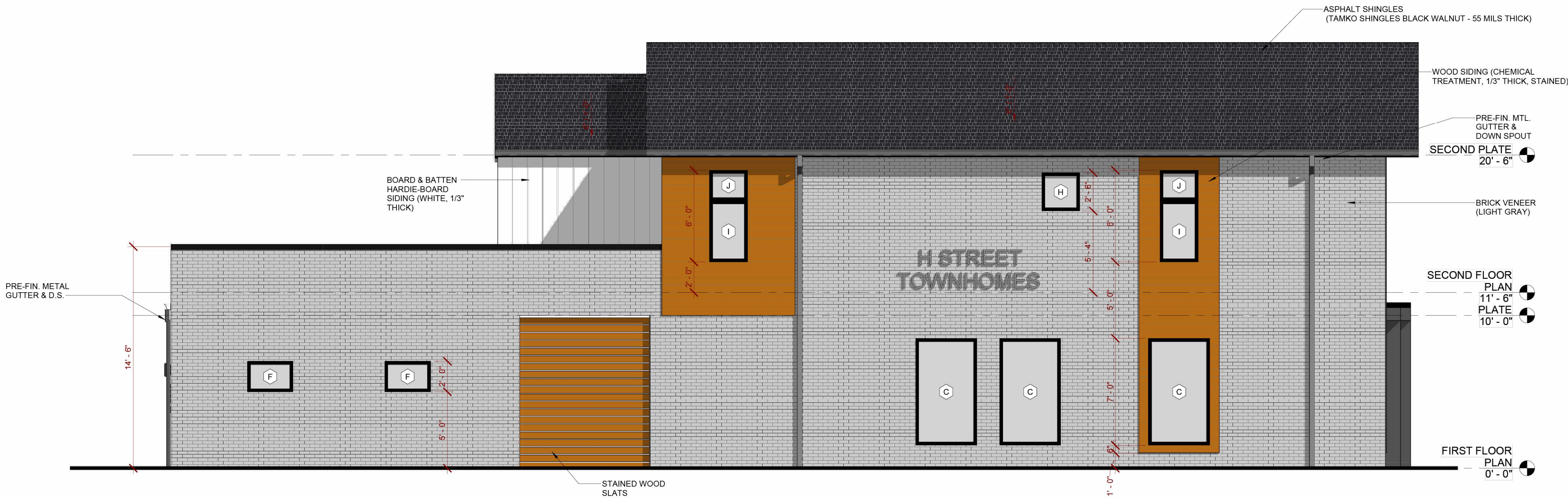
2 SIDE ELEVATION - NORTH 1/4" = 1'-0"
