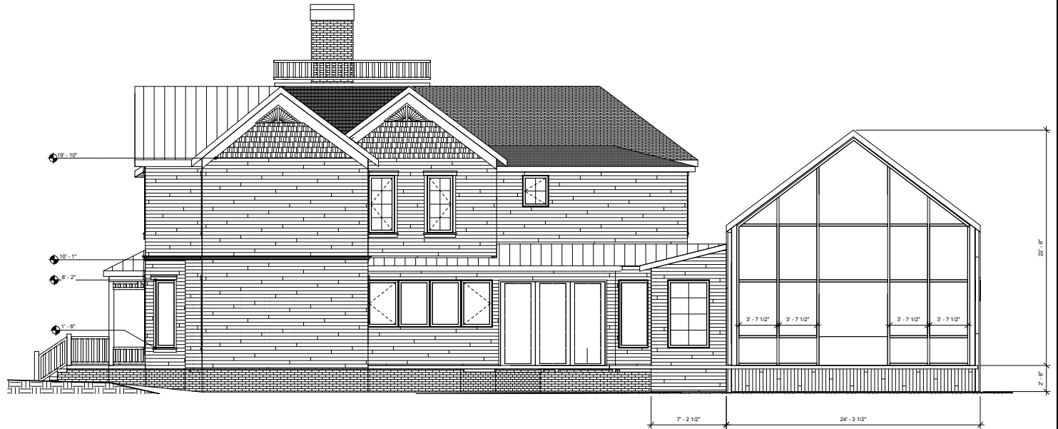
① EAST ELEVATION REMODEL 1/4" = 1'-0"
