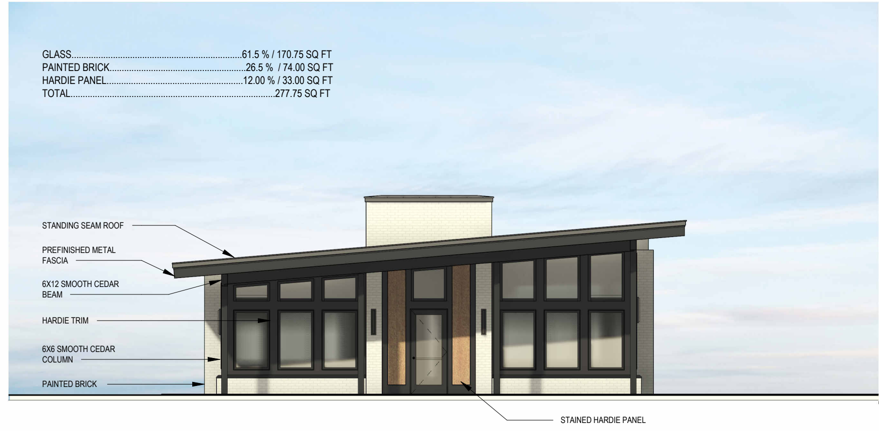
7.1 MATERIAL ELEVATIONS - FRONT ELEVATION 1/8" = 1'-0"
