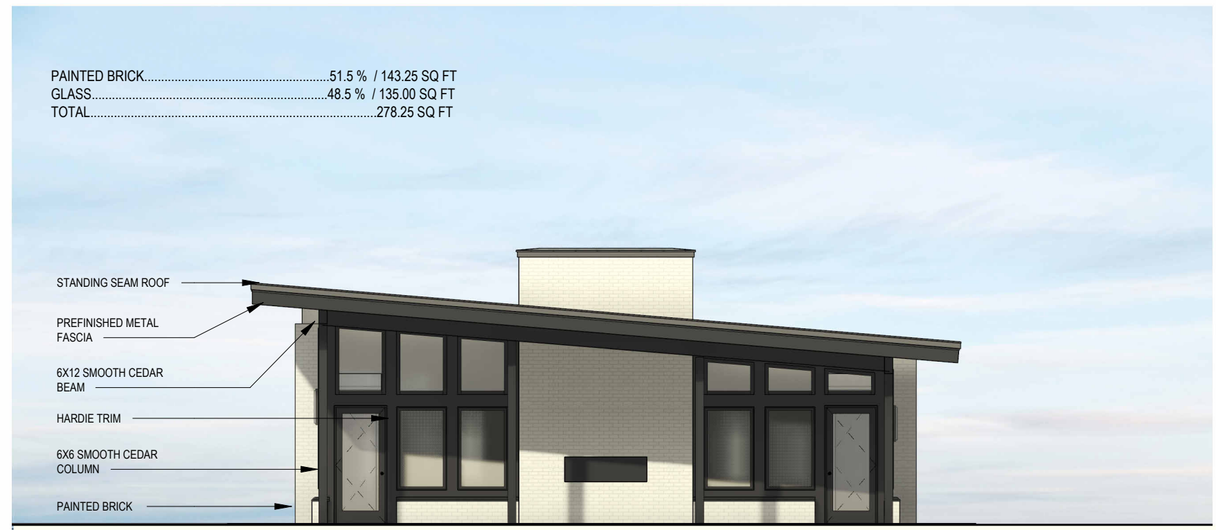
5.1 MATERIAL ELEVATIONS - REAR ELEVATION 1/8" = 1'-0"
