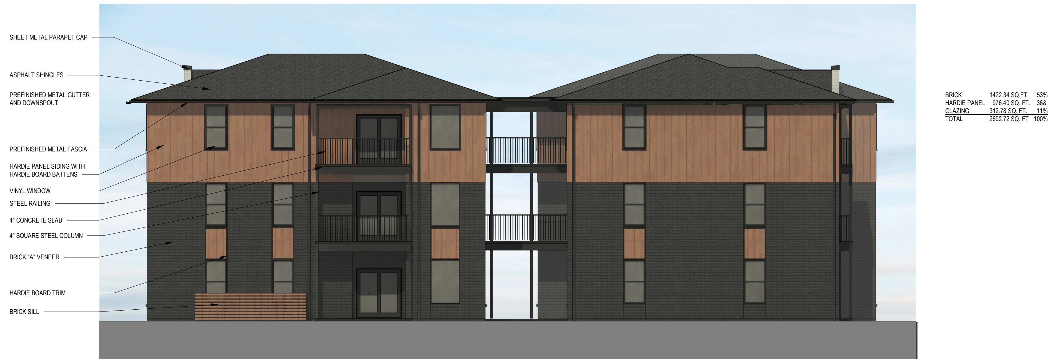
2 SOUTH ELEVATION - MATERIALS 1/8" = 1'-0"
