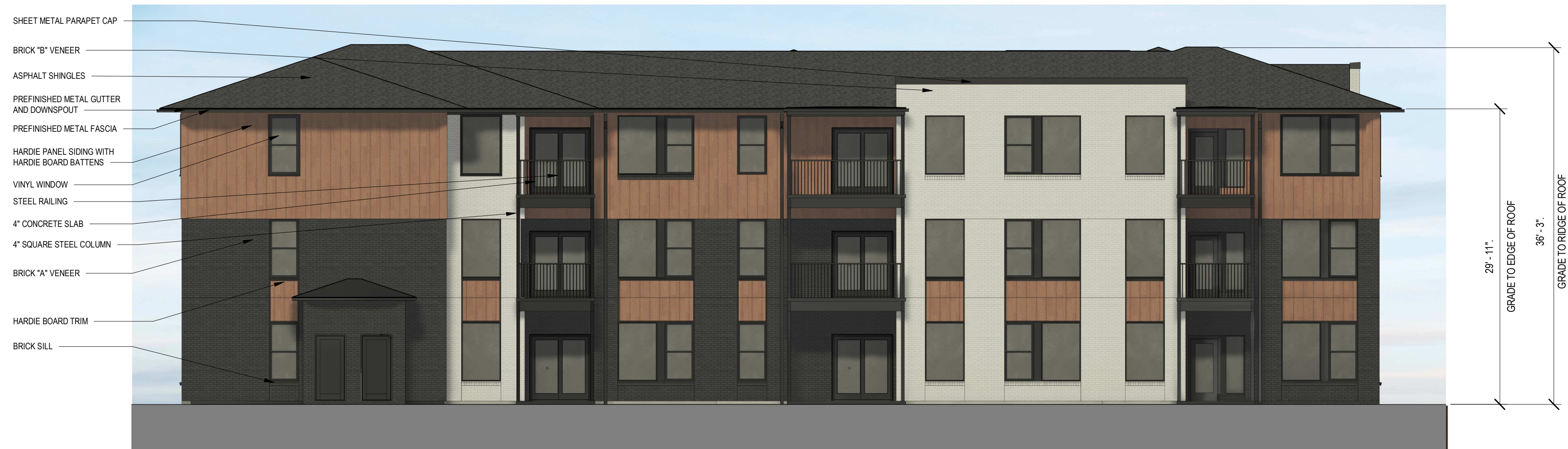
2 RIGHT SIDE ELEVATION - MATERIALS 1/8" = 1'-0"
