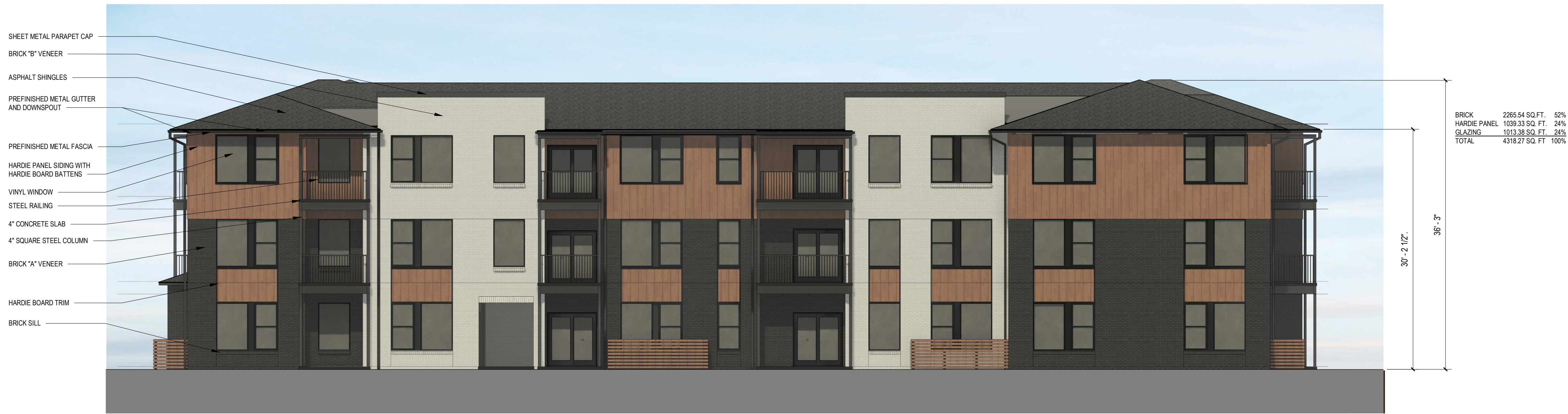
1 WEST ELEVATION - MATERIALS 1/8" = 1'-0"
