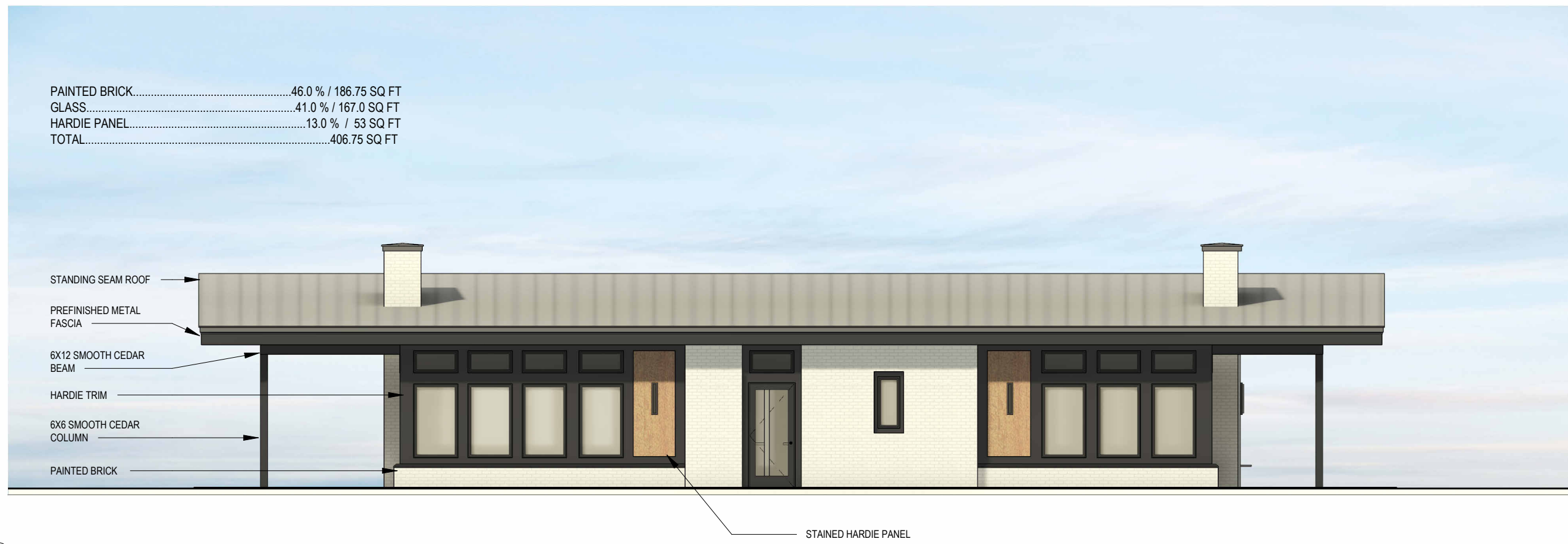
6.1 MATERIAL ELEVATIONS - SIDE ELEVATION B 1/8" = 1'-0"
