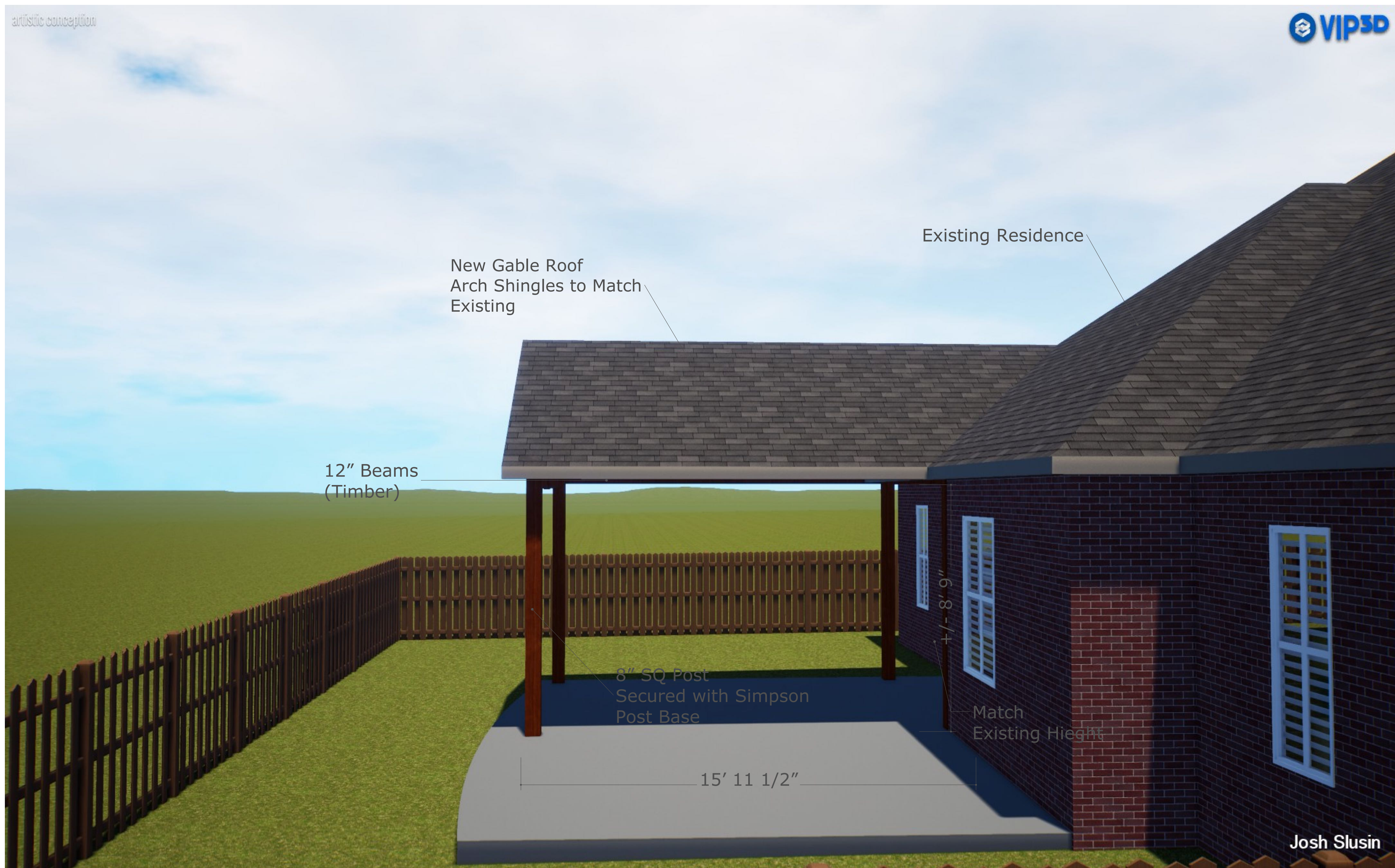
Side (East) Elevation (West Elevation Similar)
