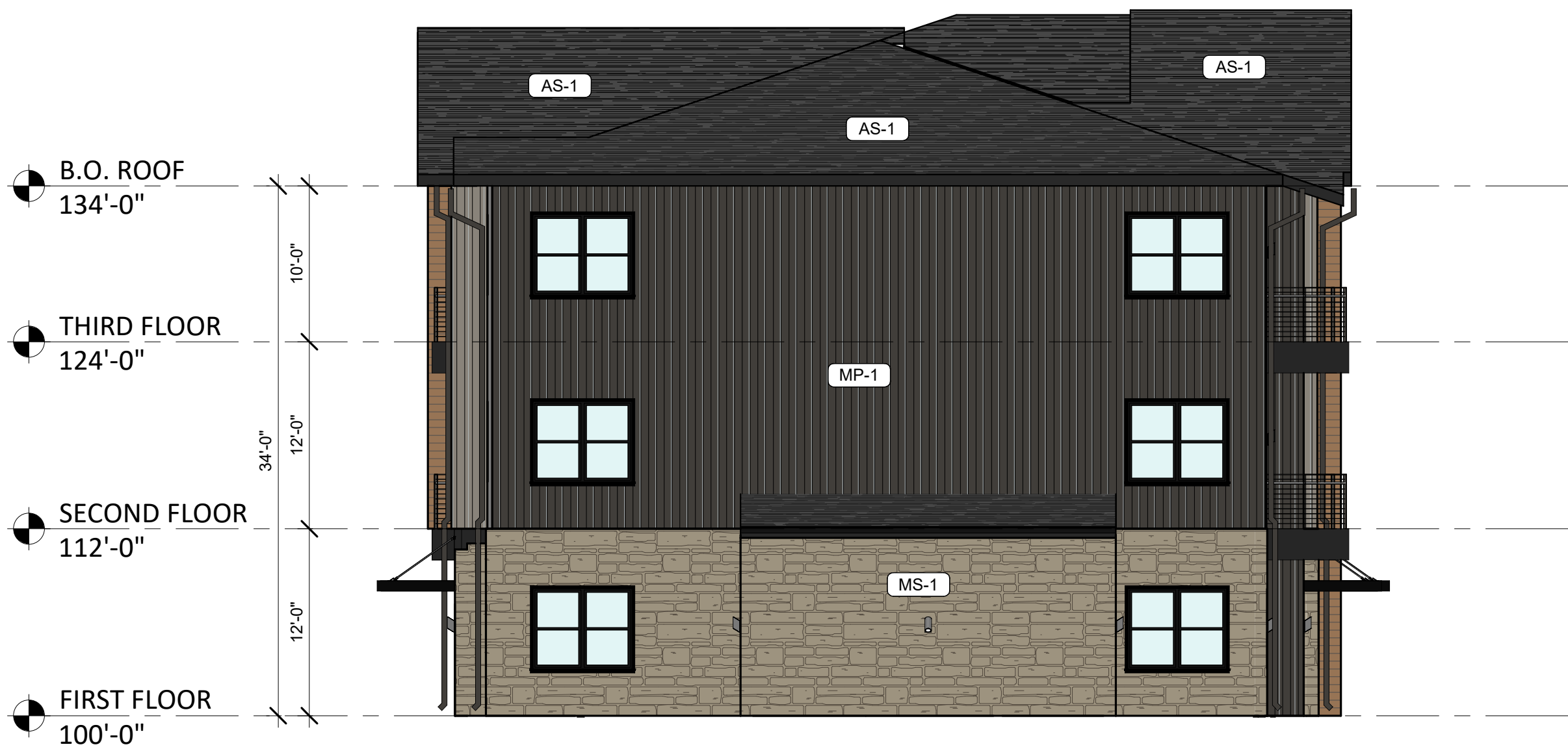
1 BLDG C_EAST ELEVATION 1/8" = 1'-0"
