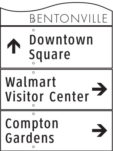
1/4" thk. aluminum panel with applied reflective vinyl graphics, mechanically fastened, SITELINK TRAC nuts
