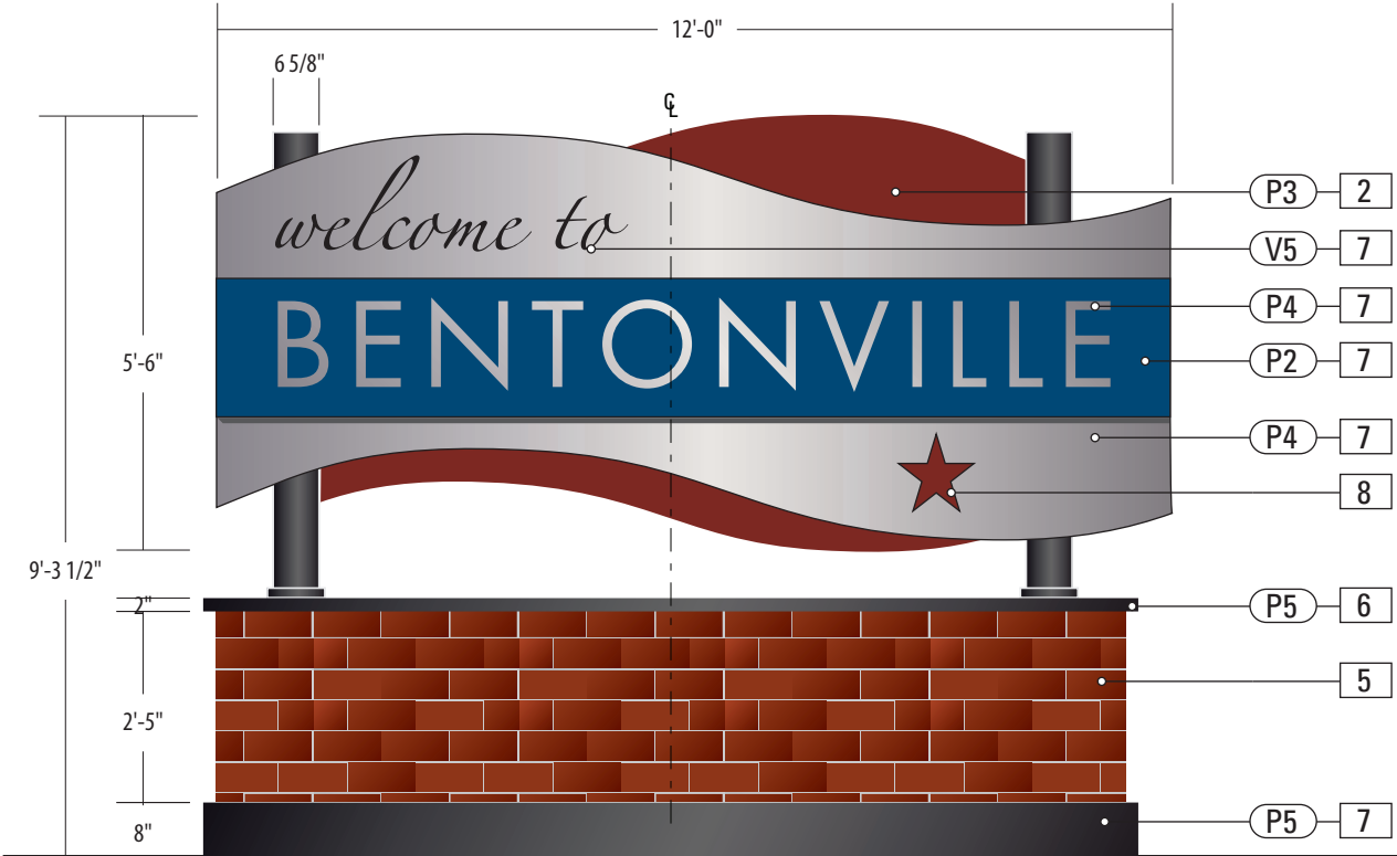
1 Front View: GATE.1a SCALE: 3/8" = 1'-0"
