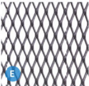
EXISTING EXPANDED METAL MESH MINIMUM 24 GAUGE
