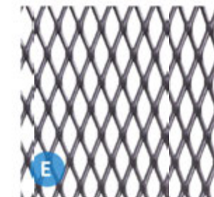
E EXISTING EXPANDED METAL MESH MINIMUM 24 GAUGE
