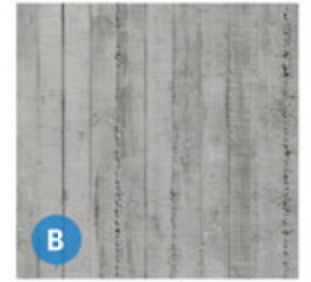
B BOARD FORMED CONCRETE
