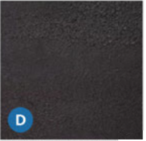
PAINTED STEEL PANEL MINIMUM 24 GAUGE
