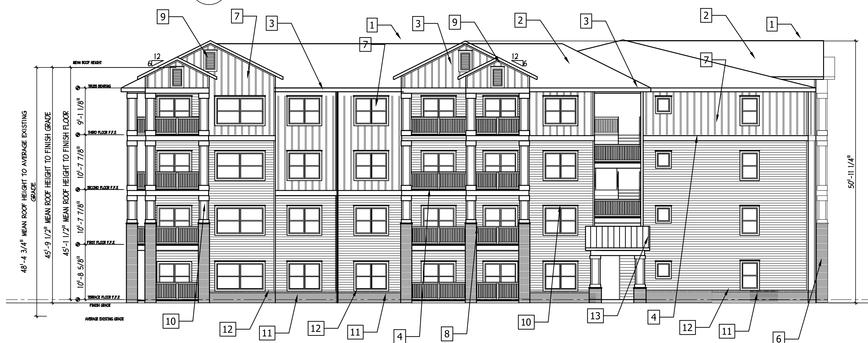
2 BUILDINGS #4 PARTIAL FRONT ELEVATION A5.2 SCALE: 3/32" = 1'-0"
