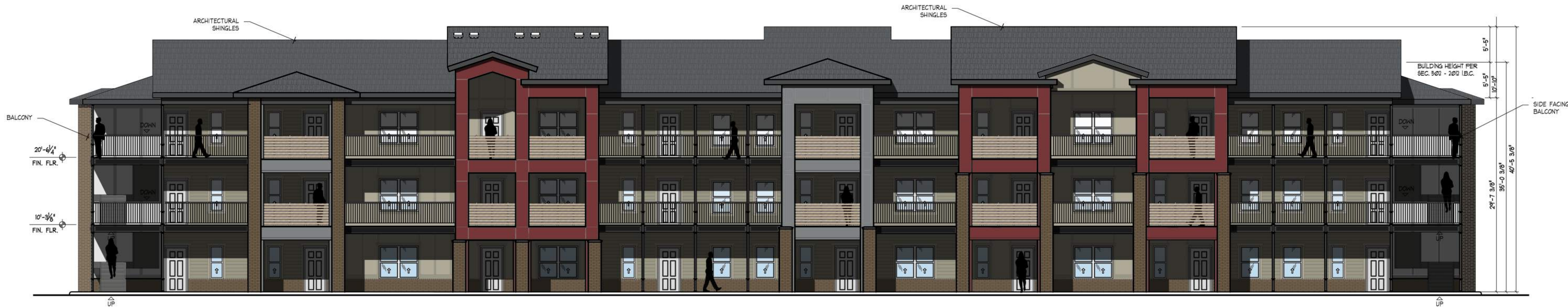
EXTERIOR ELEVATION at FRONT Scale : 1/8"=1'-0"
