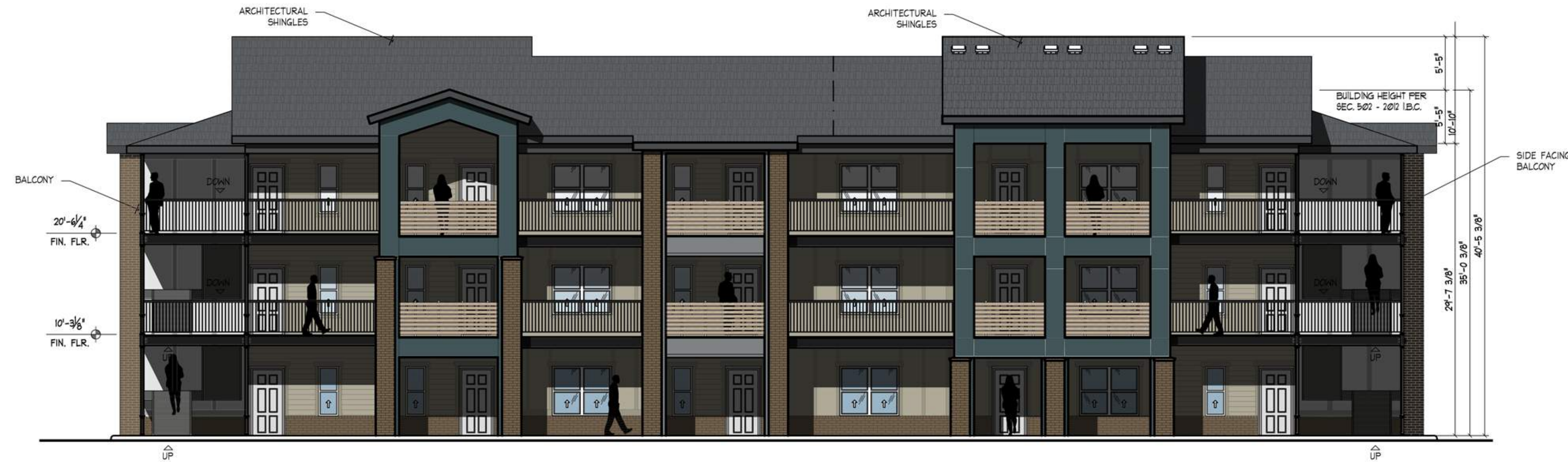
EXTERIOR ELEVATION at FRONT Scale : 1/8"=1'-0"
