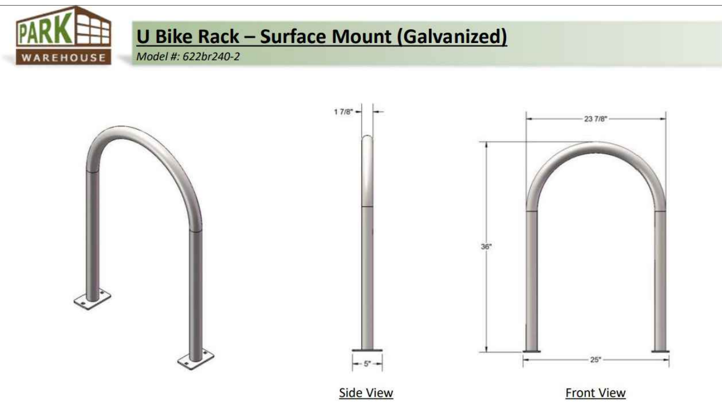
DETAIL 26 - APBP APPROVED BIKE RACK NOT TO SCALE
