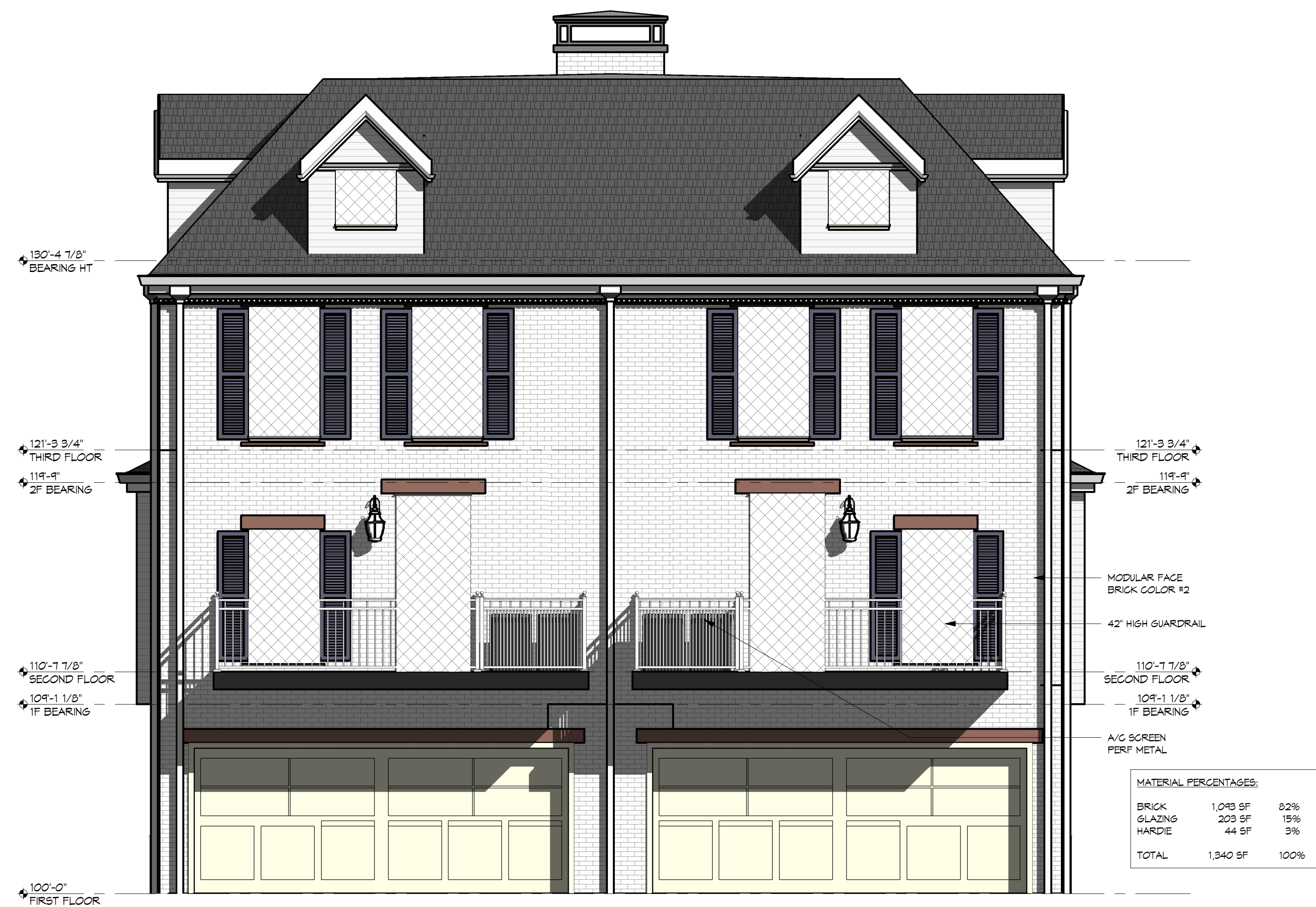
3 DUPLEX 1 - PARKSIDE - SOUTH ELEVATION 1/4" = 1'-0"
