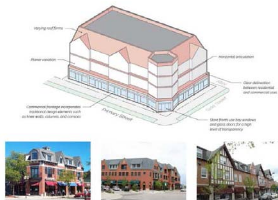
Figure 401.7-B (17) Mixed-use Design Standards
