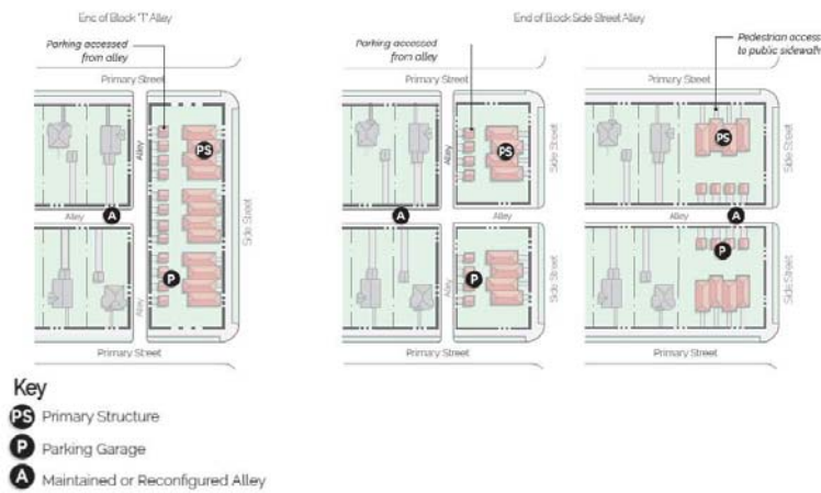
Figure 401.7-B (11) Townhouse Pedestrian & Vehicle Access - END OF BLOCK
