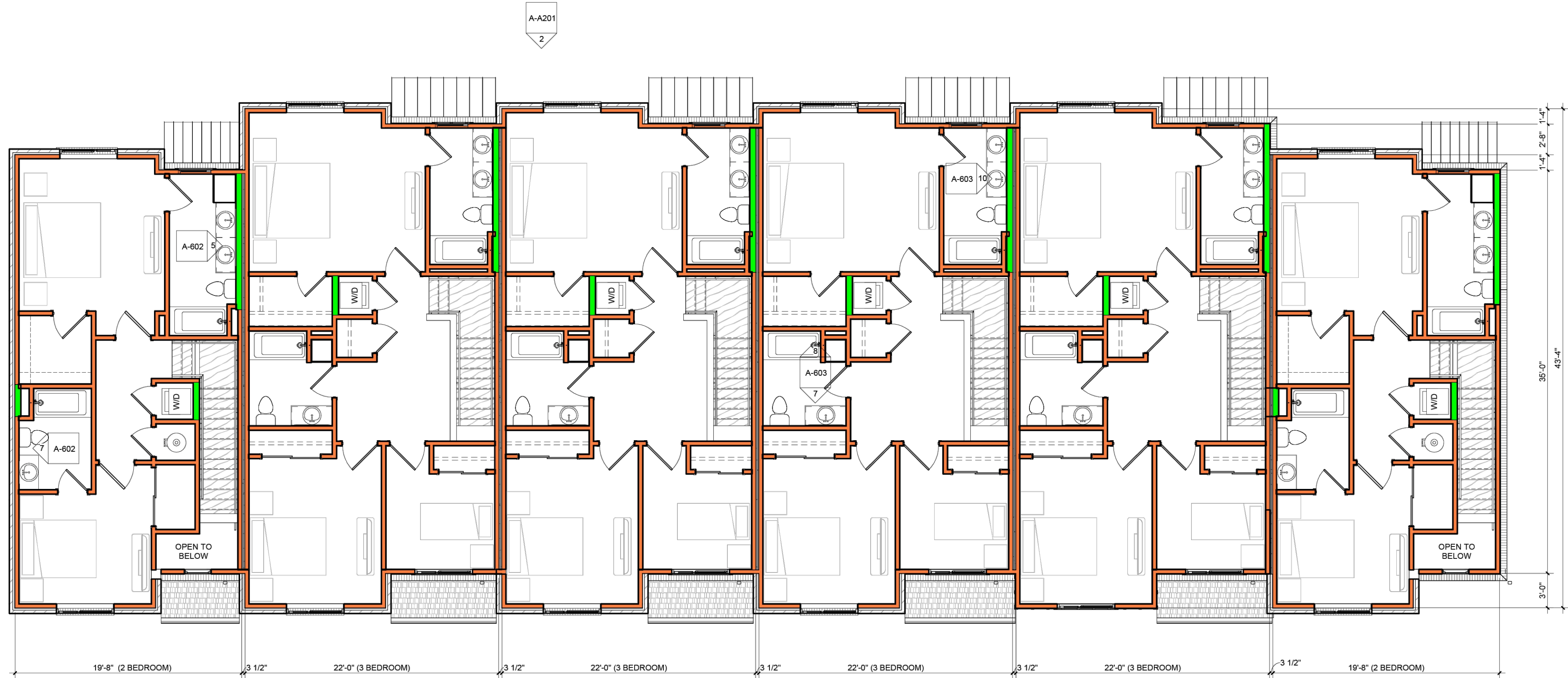
2 SECOND FLOOR - BLDG TYPE A 3/16" = 1'-0"
