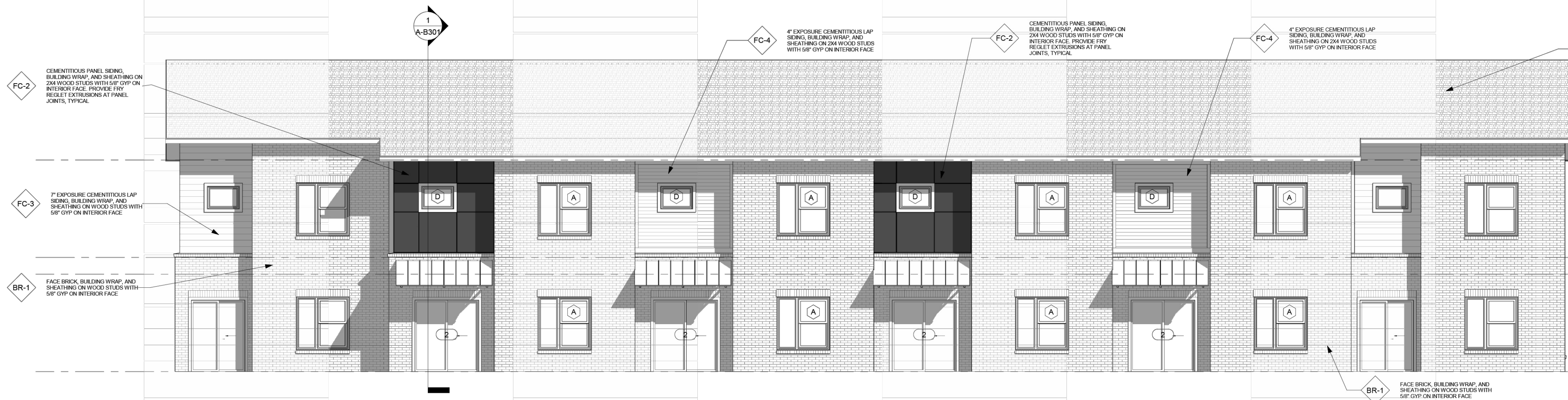
2 REAR ELEVATION - TOWNHOME TYPE 1B SCALE: 3/16" = 1'-0"
