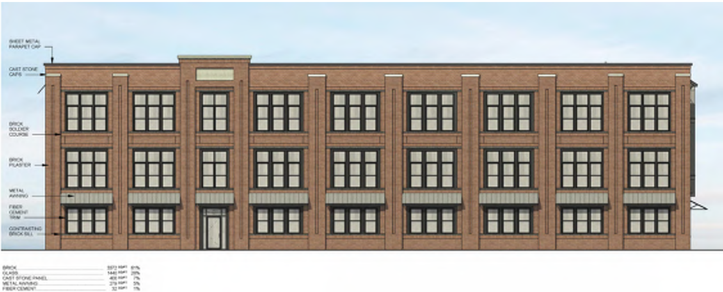
Building A - East Elevation
