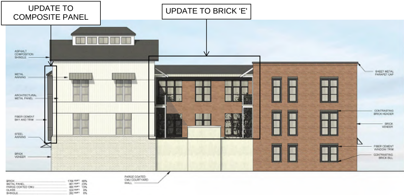
Building A - South Elevation
