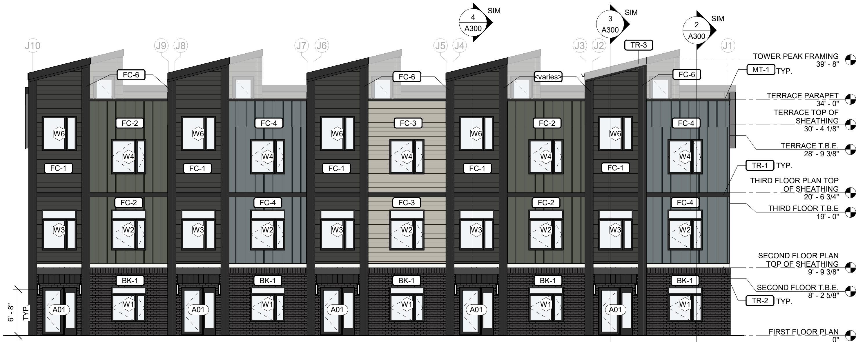
1 BUILDING TYPE 6 - "FRONT" ELEVATION 1/8" = 1'-0"
