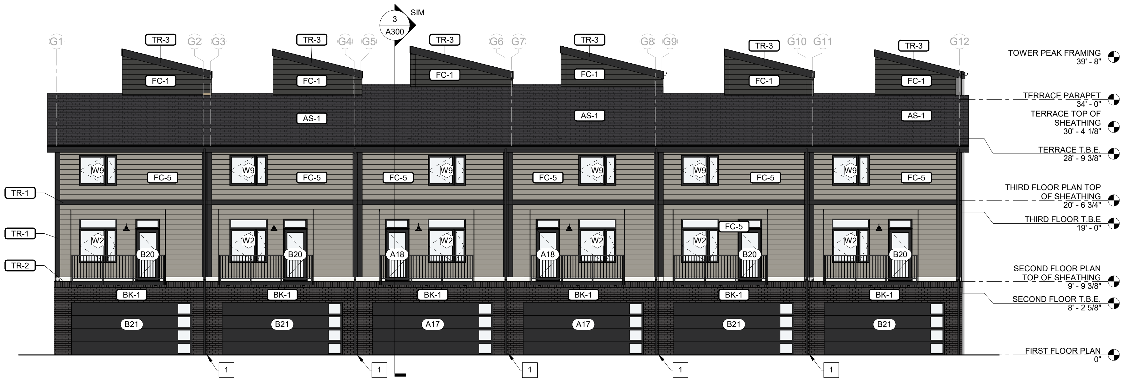
3 BUILDING G1 - "REAR" ELEVATION 1/8" = 1'-0"
