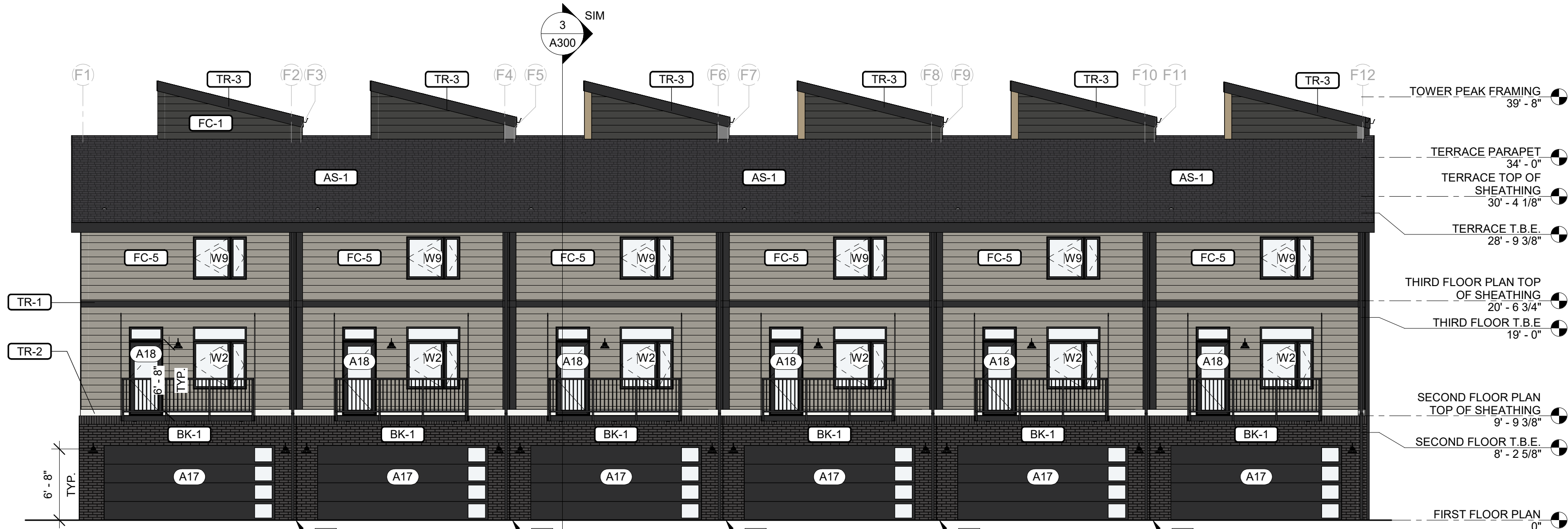
3 BUILDING TYPE 4 - "REAR" ELEVATION 1/8" = 1'-0"
