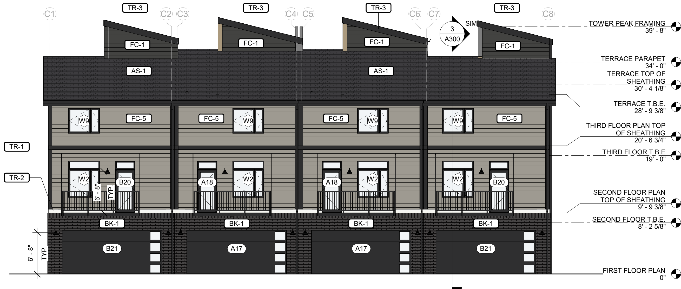
3 BUILDING C2 - "REAR" ELEVATION 1/8" = 1'-0"
