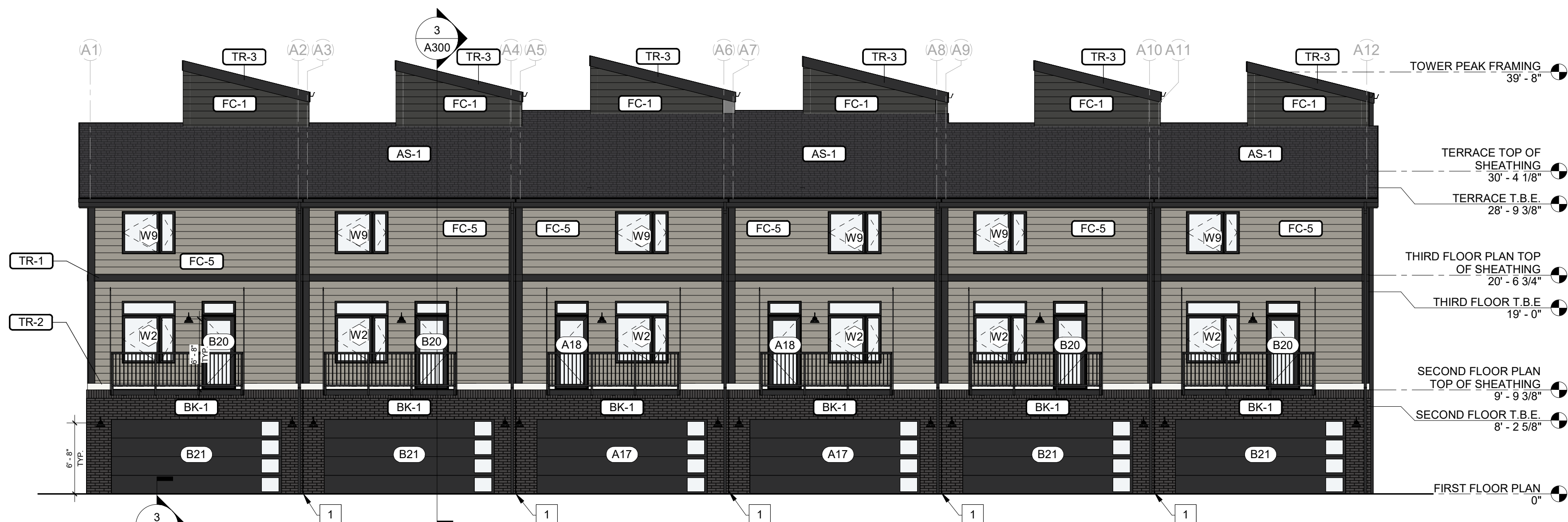
3 BUILDING A1 - "REAR" ELEVATION 1/8" = 1'-0"
