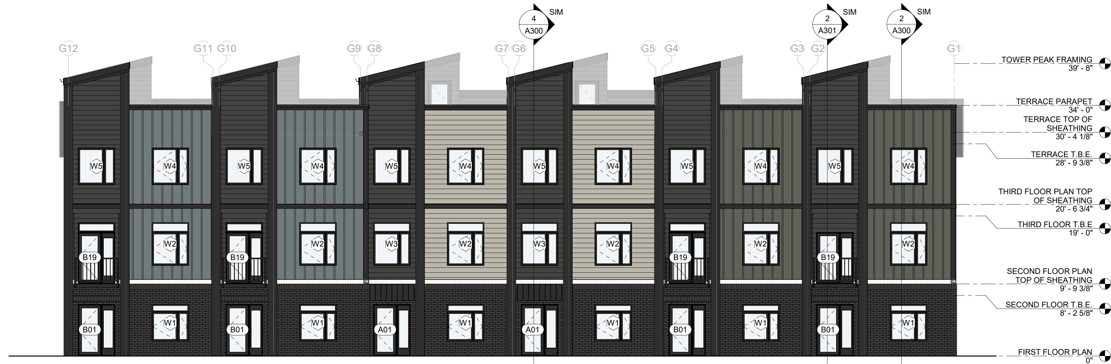
1 BUILDING G1 - "FRONT" ELEVATION 1/8" = 1'-0"
