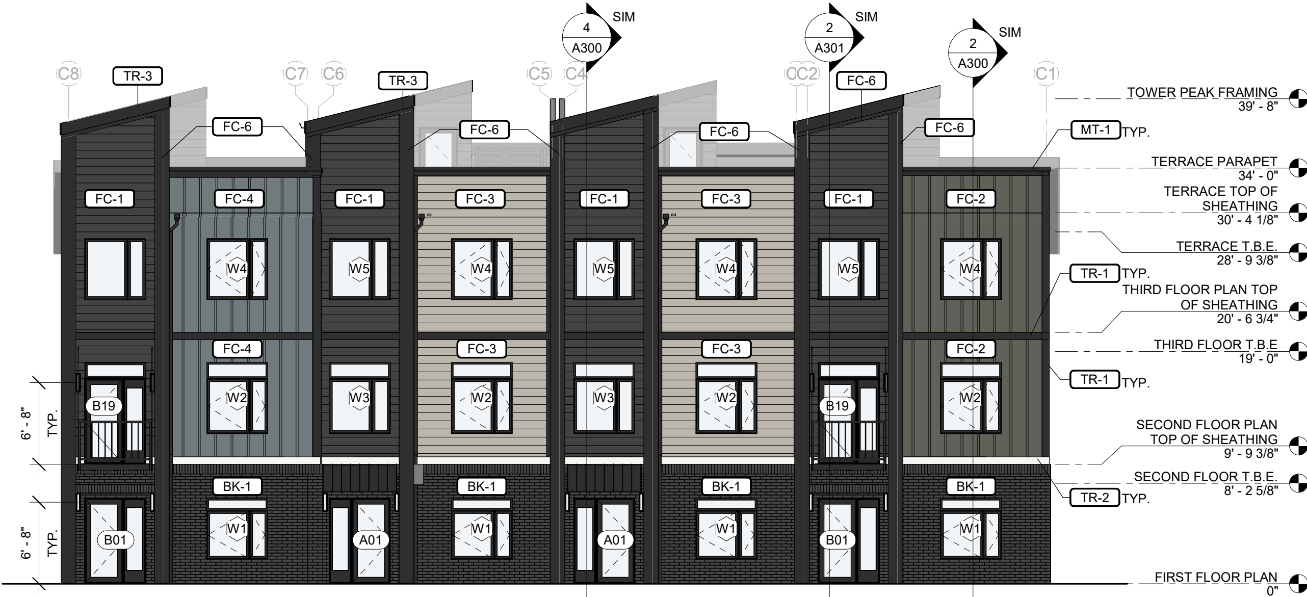
1 BUILDING C2 - "FRONT" ELEVATION 1/8" = 1'-0"
