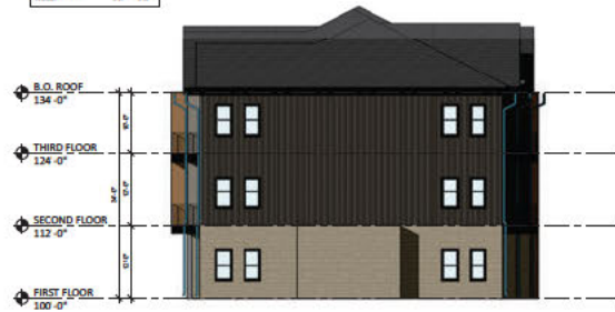
BUILDING C - EAST ELEVATION
