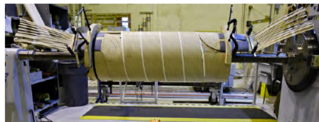
Fully Distributed Regulating Voltage Winding
