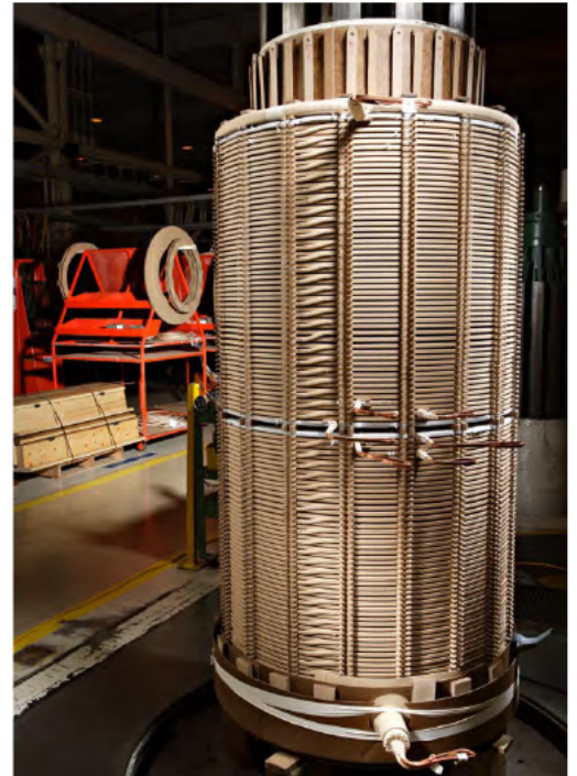
Continuous Disk Winding with Copper Magnet Wire
