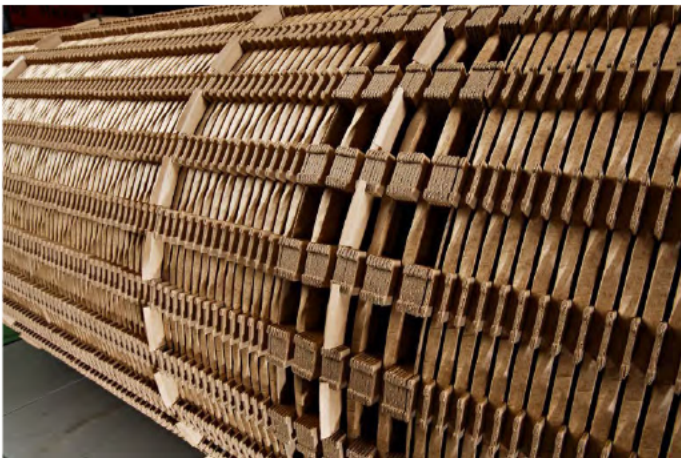
Helical Winding with CTC
