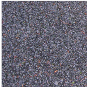
A flexible material that allows water to pass through the pavement.
