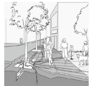
Narrow trenches in compacted subgrade to channel root growth.
