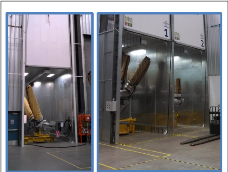
Production Testing (Shown with Chamber Doors Open) 362kV (Left), 145kV (Center), 72.5kV (Right)
